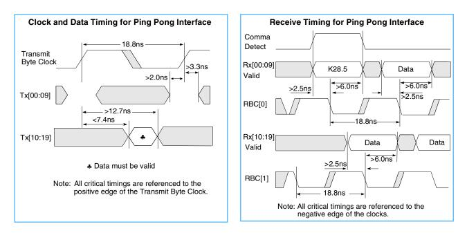
Rx[00:09] is timed off of RBC[0] as shown in the IBM42M10LCYAA20 portion of the OFC Timings on page 23. Rx[10:19] is timed off RBC[1] using identical timing specifications as in Receive Data (Rx[00:19]) on page 9. The skew between RBC[0] and RBC[1] shall not exceed  $\pm$  1.5ns.
